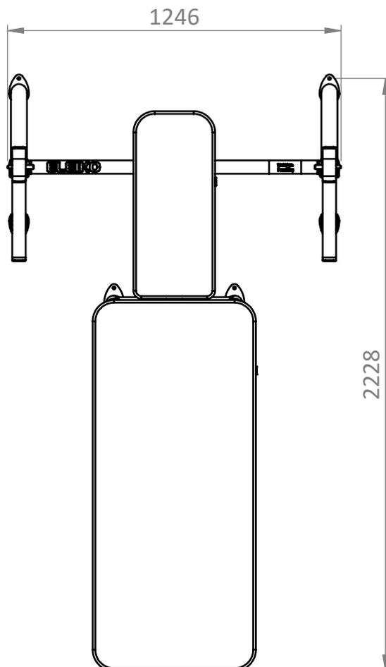
Add sufficient clearance, not less than 0,6 m, on all sides. Taking into account the accessibility to remove and replace bar and weights.
