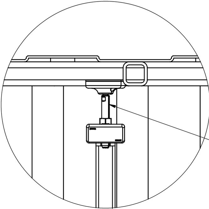
Tighten the screw (Ceiling fastener) to the container ceiling.
